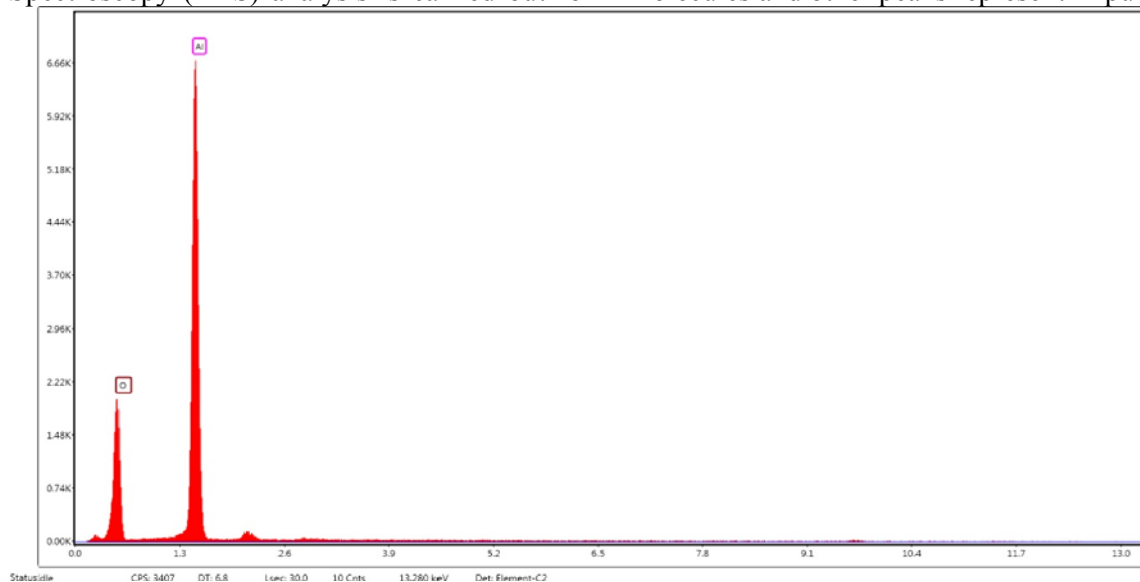
Figure 2 Energy – Dispersive X-ray Spectroscopy image of \text{Al}_2\text{O}_3 nanoparticles
