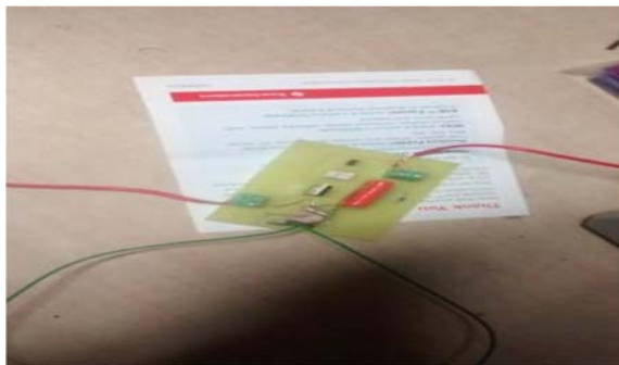
Fig [2b] PCB of Power Controlling Switch.
