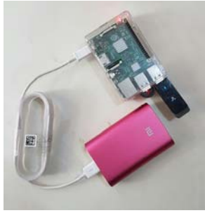
Fig. 3. Raspberry pi with a Bluetooth dongle acting as the receiver.
