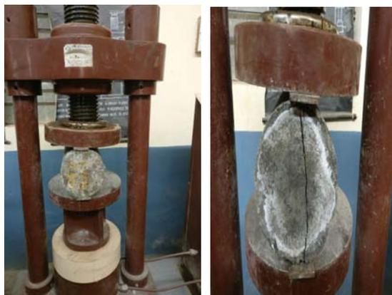
Figure 5. Split Tension Test
