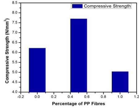
Figure 2. Compressive Strength (7 days) with fibres
