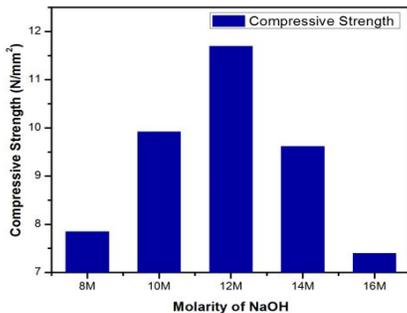
Figure 1. Compressive Strength (28 days) of different molarity
