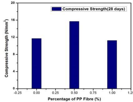
Figure 3. Compressive Strength (28 days) with fibres
