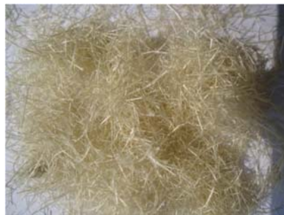
Fig 4 Fiber washed in distilled water and HCL solution
