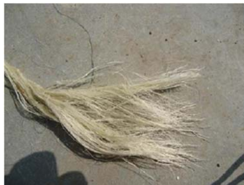
Fig 2 Extracted jute fiber
