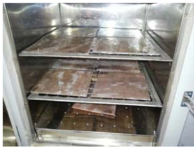
Fig 10 The specimens are dried in oven
