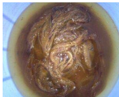
Fig 4 Fiber washed in distilled water and HCL solution
