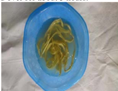
Figure 3 Fiber soaked with 10 % NaOH solution
