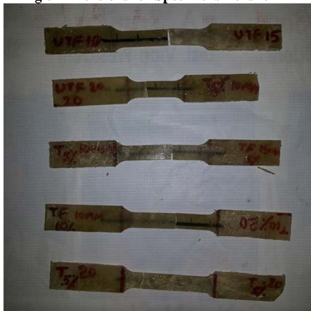
Fig 9 Tensile Test Specimens after Testing
