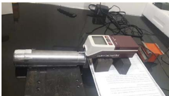
Fig(e):Conducting Surface Roughness test on the specimen.
