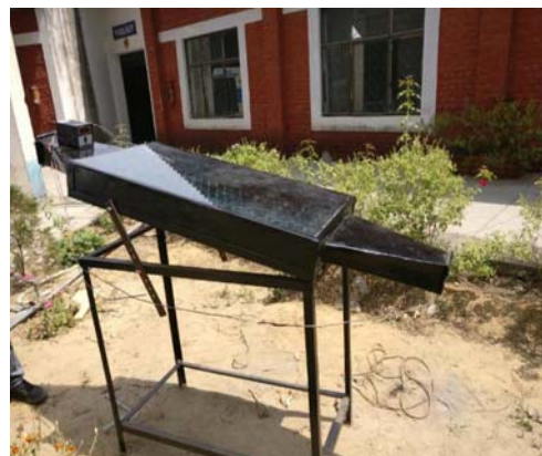
Figure 1 (a) Experimental set-up of solar air heater
