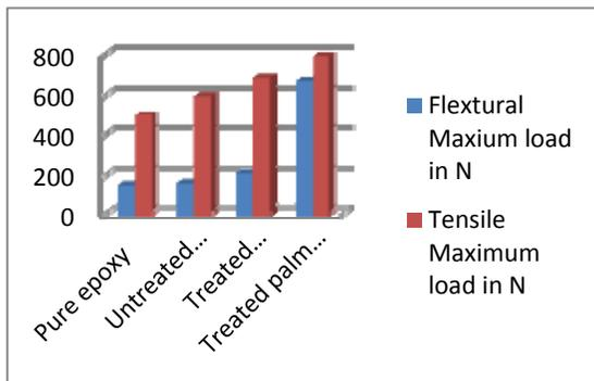
Graph-8: Flexural and Tensile Maximum load
