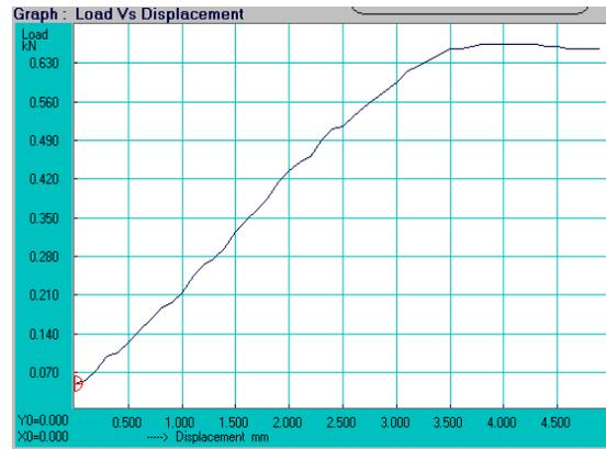
**Graph-4: Treated palm long Fiber Mat TENSILE TEST**
