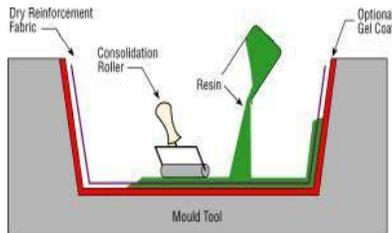
**Fig-4: Hand Lay-up Technique**
