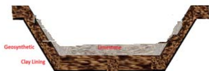
Figure 6: Diagram of Typical Successive Alkalinity Producing Systems (SAPS)
