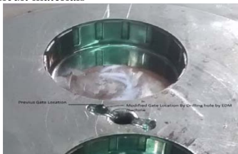
Fig9.Modified Gate Location by drilling Hole By EDM Machine
