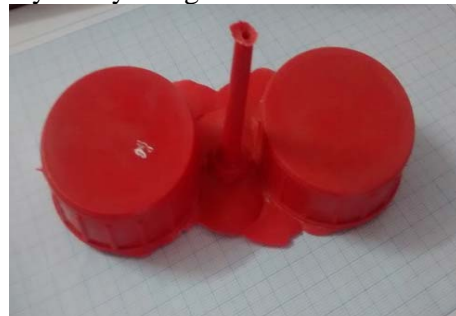
Fig2A. Defects in pressure reducer Part
