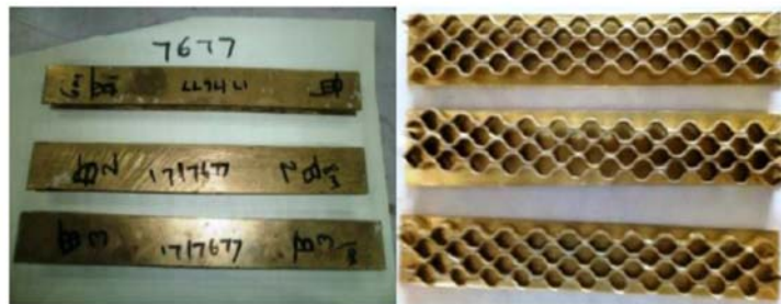
Figure (b) Sandwich Panels
