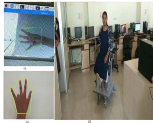
Figure.10. Gesture of four fingers, wheel chair turns left: (a) LCD displaying the gesture of four fingers, (b) alternative finger gesture, (c) Wheel chair turning towards left
