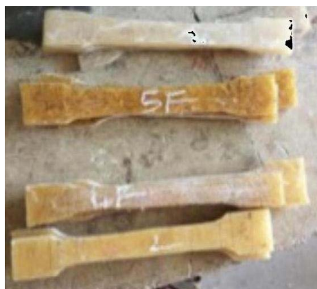
Fig2: Sample for tensile testing
