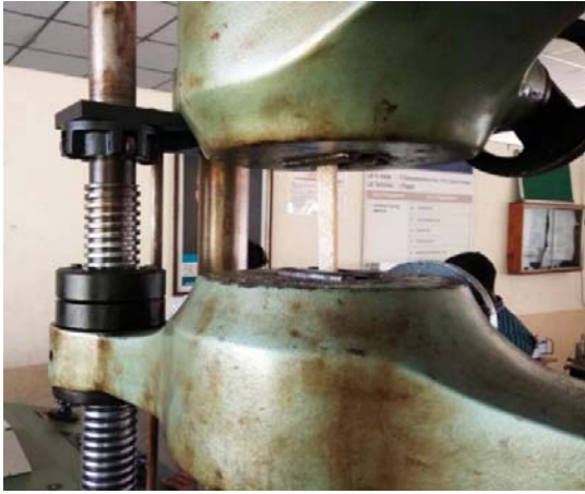
Fig3: Specimen loaded for testing on UTM
