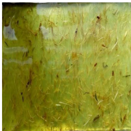
Fig1: Fabrication procedure of bagasse embedded epoxy composite
