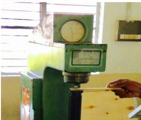
Fig 5: Hardness test on Rockwell Hardness Apparatus
