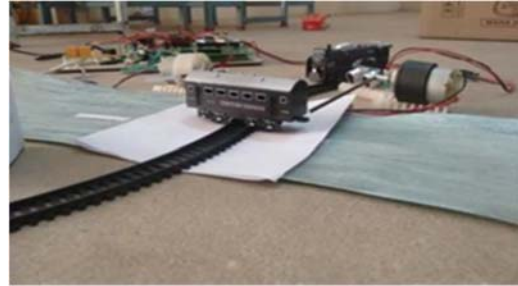
Figure 8. Ultrasonic sensor checks for obstacle after closing the gates
