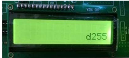
Figure 9. LCD continuously displays the distance between ultrasonic sensor and constant obstacle
