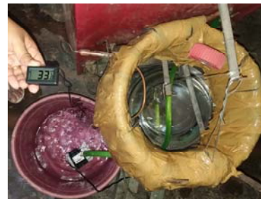
Fig. 4 Condenser Tube with Insulation
