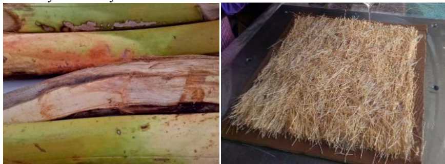
Fig. 2.3. Pictorial view of (a) Coconut bunch fiber source and (b) Coconut bunch fiber.
