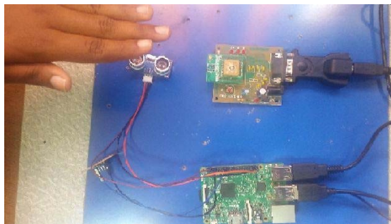
Fig. 5. Prototype for detection of objects in the railway track.
