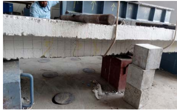
Fig 5. Final Failure In Beams By Crushing Of Concrete
