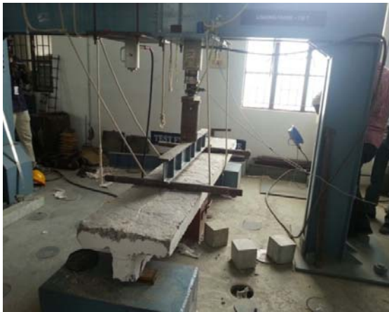
Fig 4. Test Setup of T-Beam
