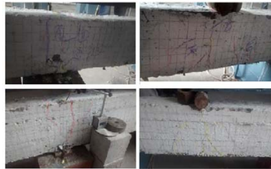
Fig 7. Final Failure In Beams By Crushing Of Concrete
