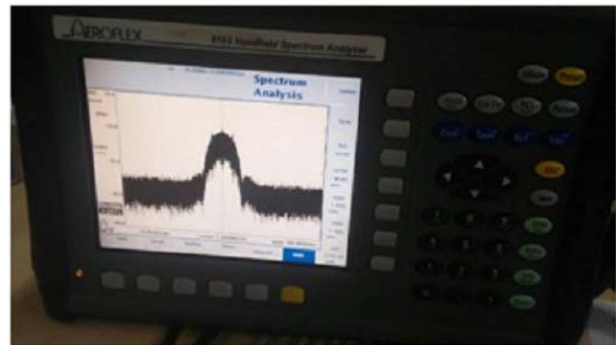
Fig.7 The Final output DSSS waveform on Spectrum Analyser
