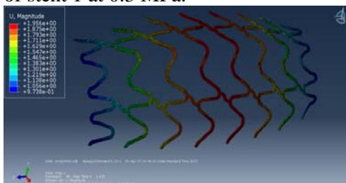
Fig-4.14 Maximum and minimum deformation of stent 1 at 0.4 MPa.
