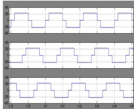
**Figure 7. Voltages waveforms of 3 level inverter fed Induction motor**
