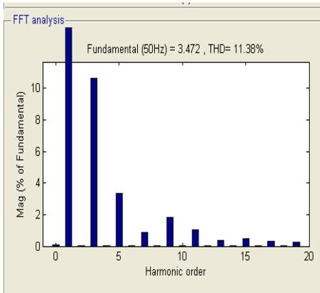
**Figure 11. FFT spectrum for stator voltage of 3 level inverter fed IM drive**
