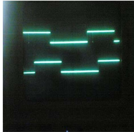
**Figure 13. Driving pulses for three level inverter circuit**
