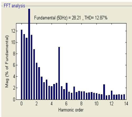
**Figure 5. FFT analysis for stator current of VSI-fed IM drive**
