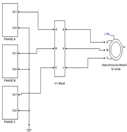
**Figure 6. Block diagram of 3 phase multilevel inverter-fed IM**
