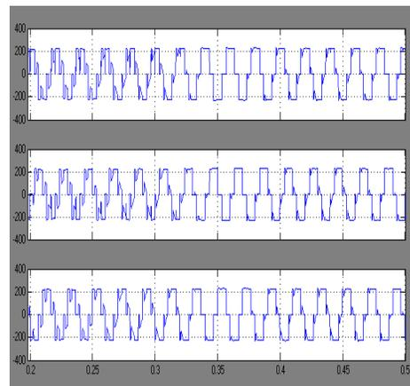
**Figure 2. Phase voltage waveforms of VSI-fed IM drive**
