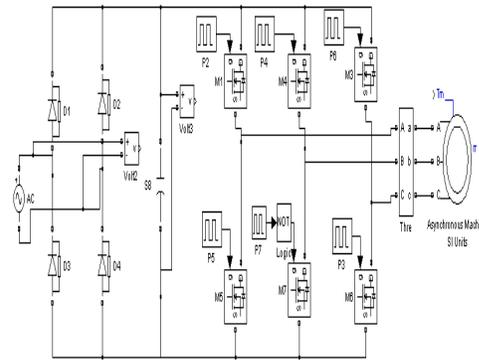
Rectifier Link filter PWM inverter
