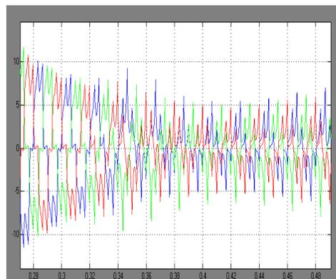
**Figure 3. Stator current waveforms of VSI-fed IM drive**
