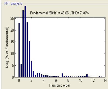
**Figure 10. FFT spectrum for stator current of three level inverter fed IM drive**
