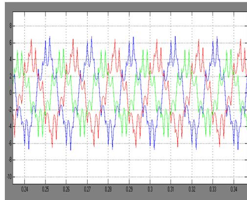
**Figure 8. Stator current waveforms of three level inverter fed induction motor drive**
