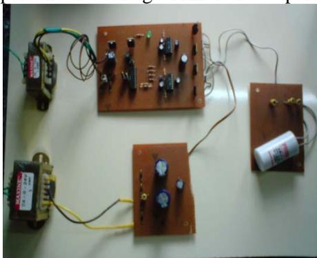
**Figure 12. Hardware snap shot of three level inverter**
