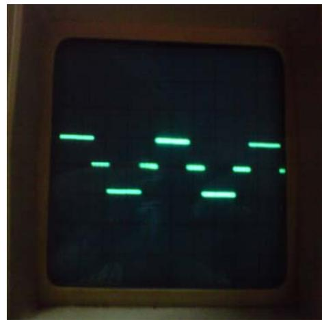
**Figure 14. Output voltage of three level inverter.**
