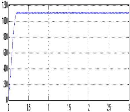
**Figure 4. Rotor speed of VSI-fed induction motor drive**
