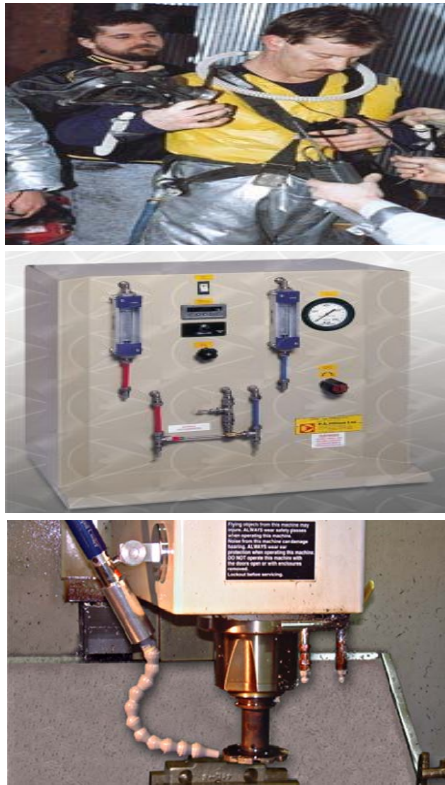
Fig.1. Basic operation of vortex tubes :(a) Air suits of Vortex tube and (b) the Vortex tube refrigerator (c) the Vortex tube Cooling System for a drill bit.
