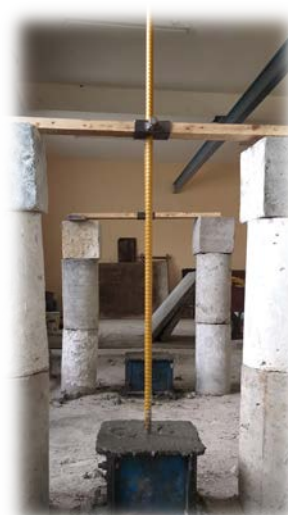
Figure 2- Casting Setup of Specimens for Pullout Test
