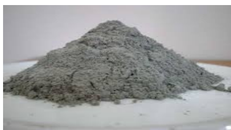
Figure 3: Sample of fly ash
