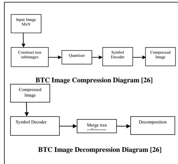
**Figure1: Diagram for Block Truncation Coding**
