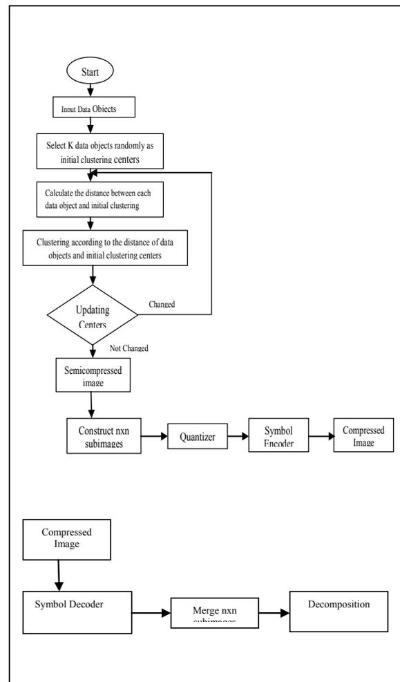
**Figure3 : Block Diagram for K-Means Clustering Algorithm and Block Truncation Coding**
