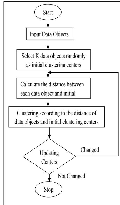
**Figure2: Block Diagram for K-Means Clustering Algorithm**
