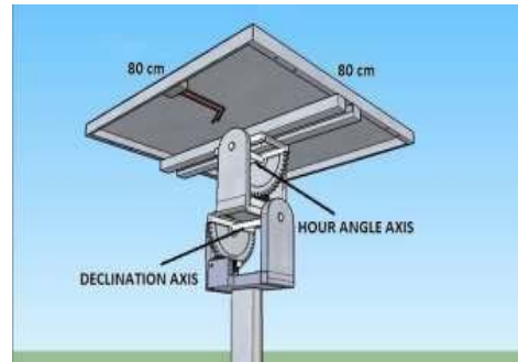
Fig.2. Mechanical structure for the dual-axis solar tracker
