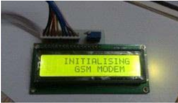
Figure 3. Hardware implementation of car security system LCD initialization
