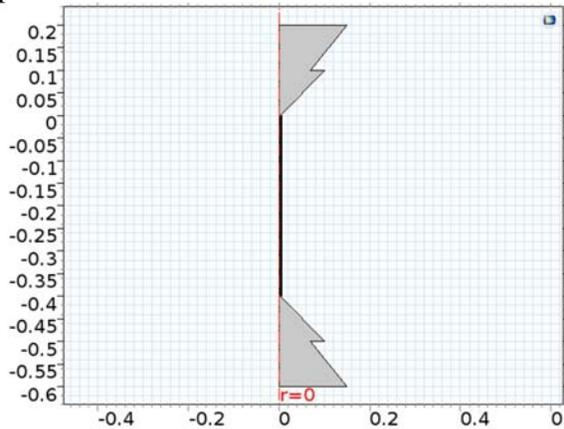
Figure .3: symmetrical half of Novel Biconical antenna.
