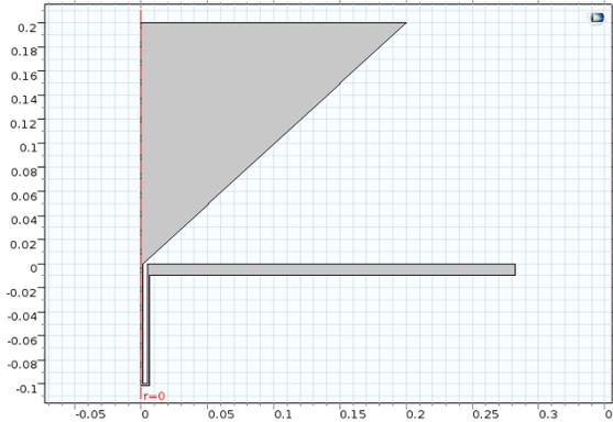
Figure 2: Symmetrical Half of Biconical Antenna.
