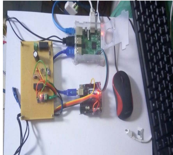
Figure.5. Implementation of Optimal Energy Management Controller for rectifying the battery charging problem
