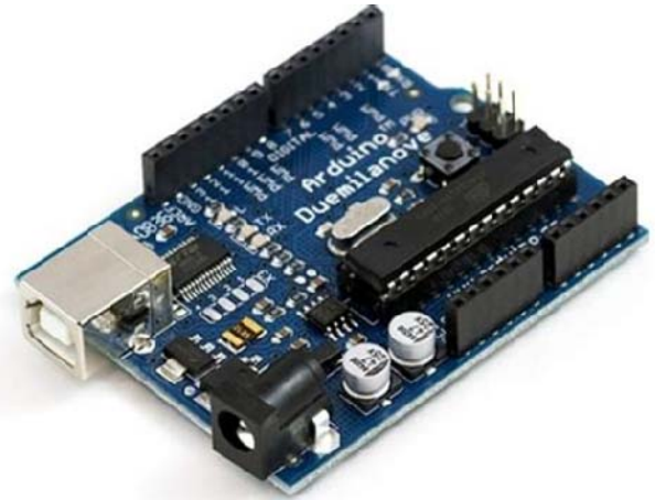
Fig.4.2 Arduino Uno microcontroller board (interface)
