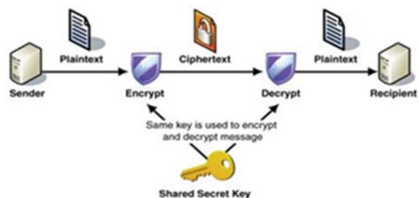
Fig. 1. Simple Encryption Scheme
