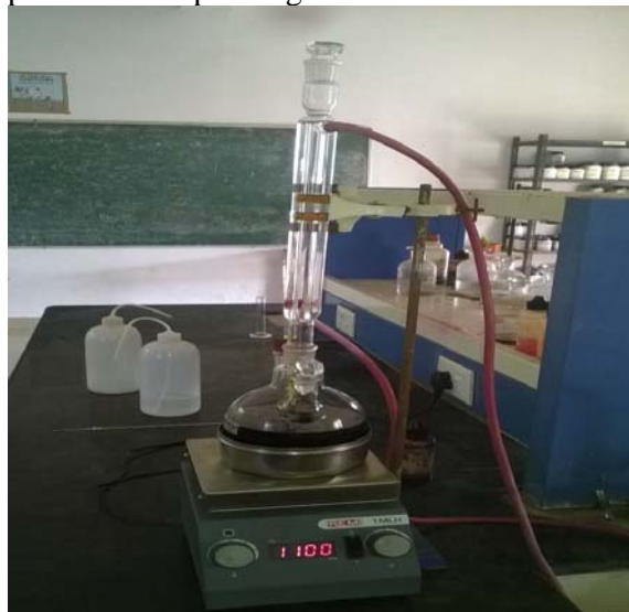
Fig.2.1 Transesterification of biodiesel
