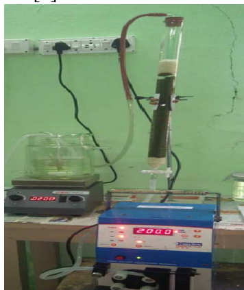
Fig.1 Column packed with Marine green algae ulva lactuaca
