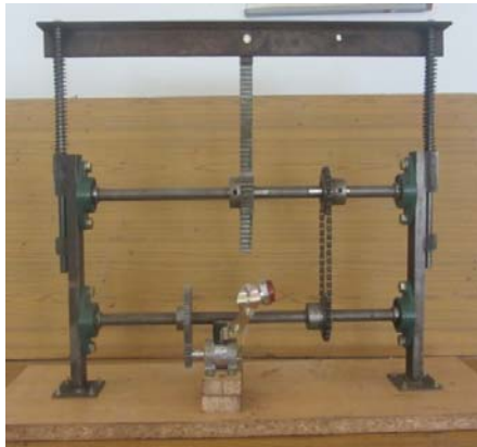
Fig: 2 Front view of the footstep electric generator
