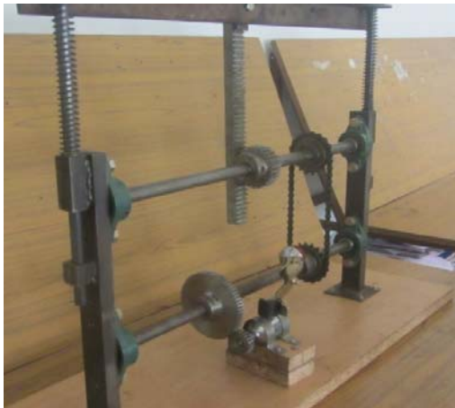
Fig 6.2 Side view of the footstep electric generator
