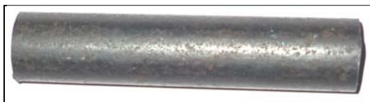
Fig .1 H13 tool steel Dia. 18 mm × 100 mm.
