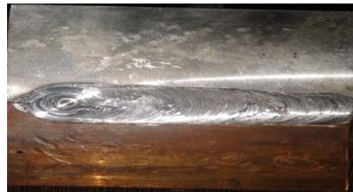
Fig.6:FSW joint of AA 2014T6 & ETP Copper
