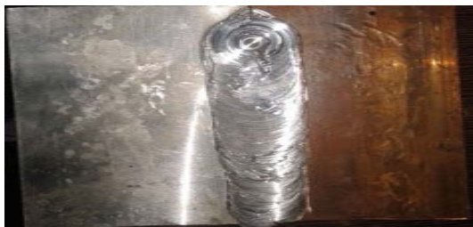
Fig.12:FSW joint of AA 2014T6 & ETP Copper
