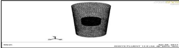
Fig: 5.Oil Reservoir with Copper Bar Mesh
