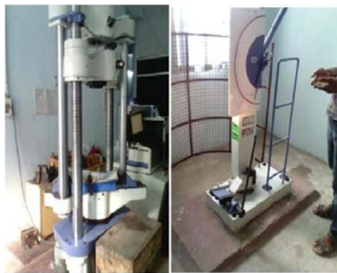
Figure3.3. Experimental set up and loading arrangement for the specimens for tensile test and impact test
