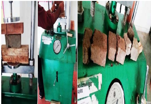
Figure 8: compression testing procedure
