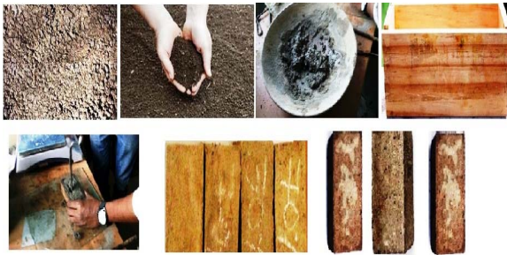
Figure 2: Clay and Paper Residue Composite Bricks
