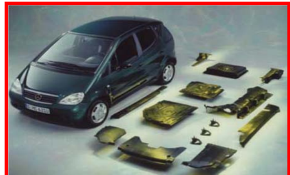
Fig 17: Interior parts of the Mercedes A-200 reinforced by natural fibers
