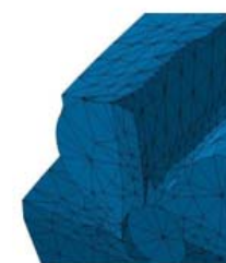
Figure 13: Deformed Mesh for Transient Dynamic Load Condition at 54°
