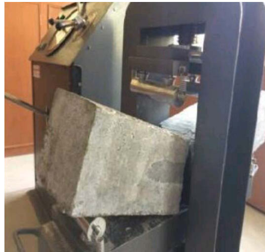
Fig 5 flexural strength of beam
