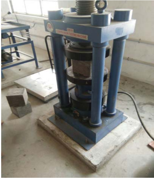
Fig-3 Compressive strength of cube
