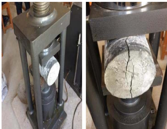
Fig-4Tensile test on cylinder
