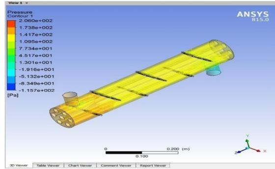
Fig.5. It shows the Heat Exchanger Temperature at the Baffle angle is placed in 45°
