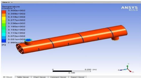
Fig.2. It shows the Heat Exchanger Temperature at the Baffle angle is placed in 90°
