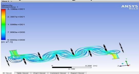
Fig.4. It shows the Heat Exchanger Fluid flow streamlines at the Baffle angle is placed in 90°
