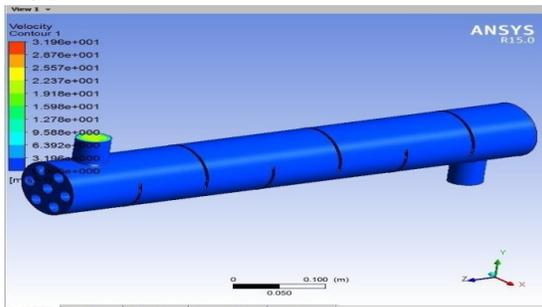
Fig.3. It shows the Heat Exchanger Velocity at the Baffle angle is placed in 90°
