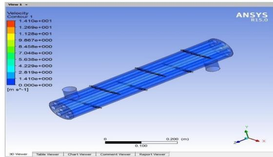
Fig.7. It shows the Heat Exchanger Velocity at the Baffle angle is placed in 45°
