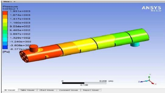
Fig.1. It shows the Heat Exchanger Pressure at the Baffle angle is placed in 90°
