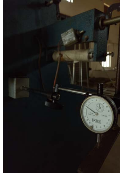
Fig 2 Deflection meter setup on UTM
