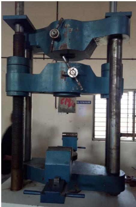
Fig 1: Pull out test setup
