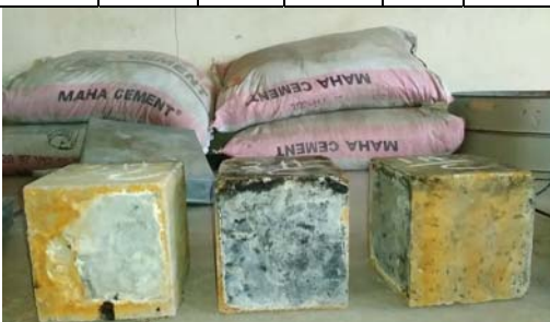
Fig. 3.6 Cubes after acidic attack (HCl)
