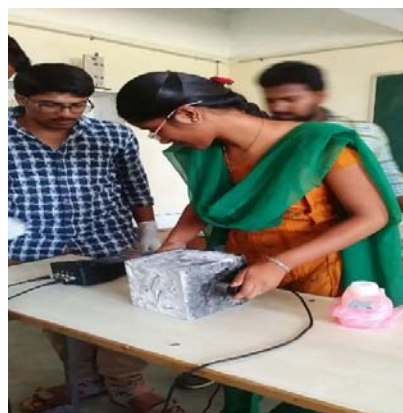
Fig.3.2 Ultrasonic Pulse Velocity test of cubes
