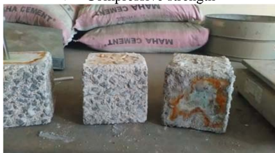
Fig.3.3 Cubes after acidic attack ( H_2SO_4 )
