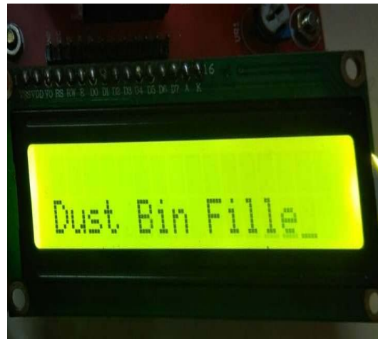
FIG 10 The message displayed on the LCD screen when the bin gets filled.
