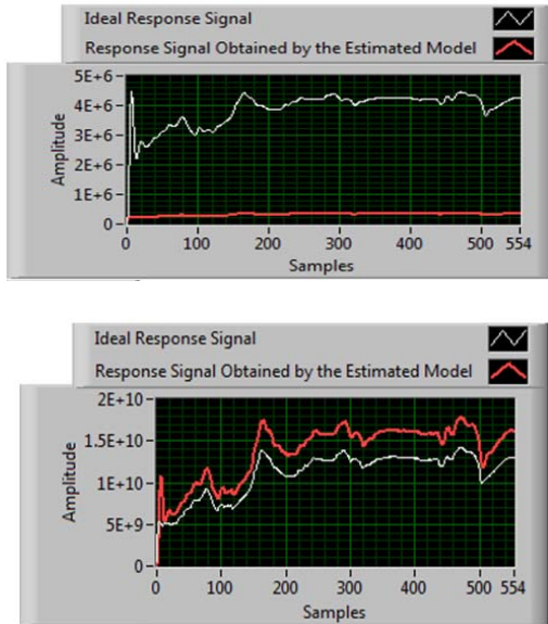
Figure 15: Response of estimated Hammerstein, wiener and wiener-Hammerstein models for steam load signal
