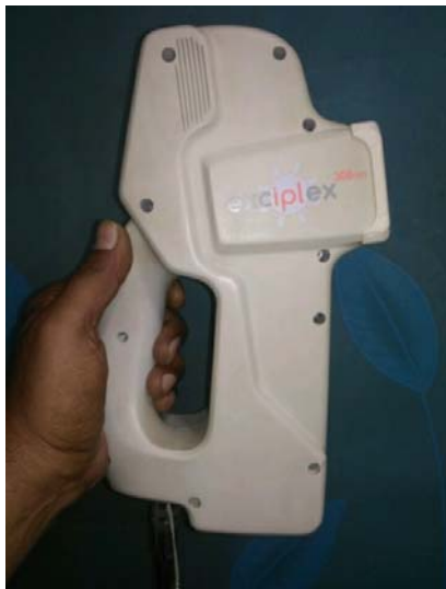
Fig.1 The exciplex excimer lamp unit with 308 nm radiation used for treatment of small patches of vitiligo.
