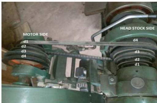
Fig 1: conventional lathe head stock equipped with stepped pulley
