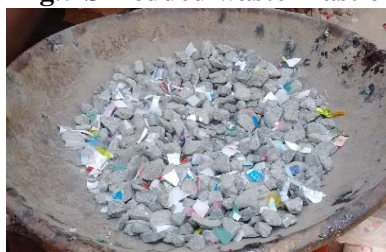
Fig.6 Shredded plastic mixing with heated aggregate
